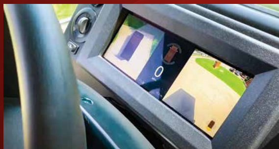
360° Camera System with Proximity Sensors
